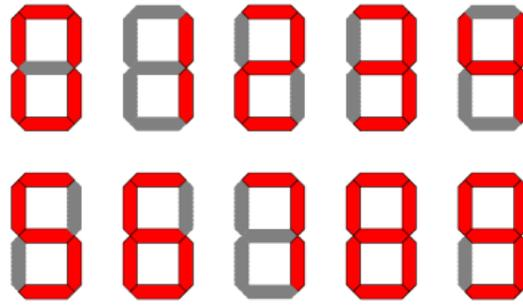
Figure 2: Patterns for generating 0-9 numbers using 7 LEDs segments
