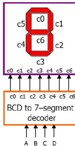
Figure 3: inputs and outputs for BCD to 7-segment display
