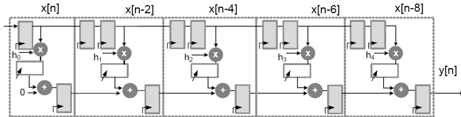
Pipeline direct form FIR filter for FPGAs with DSP48 blocks
